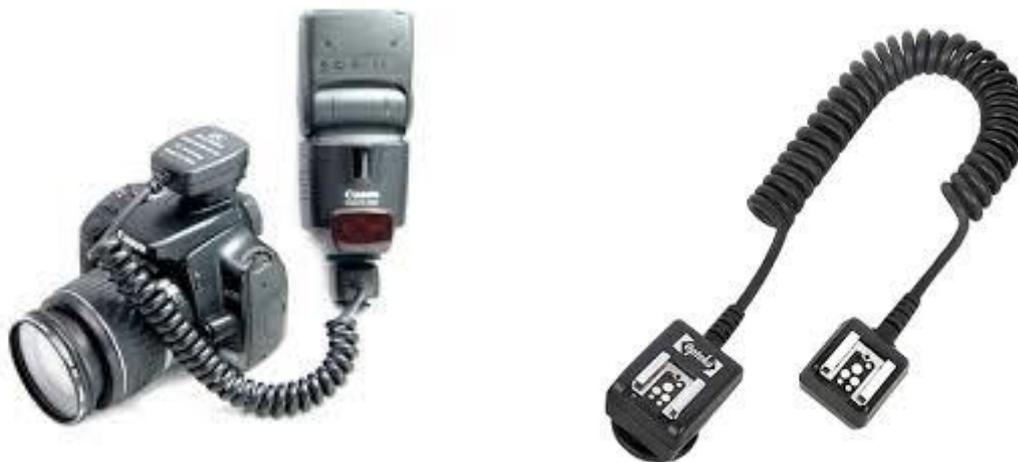
These are cables with a male and female hot shoe attachment at each end. One end connects to the camera hot shoe and the flash gun fits into the other. When the camera and flash are switched on all of the available flash and camera functions will work just as if the flash were mounted on the camera but with the benefit that the flash can be moved to light the subject better, subject to the length of the cord.
